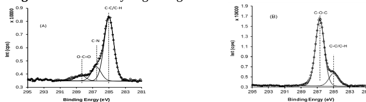
Figure 2. The XPS C 1 s spectra of (A) PEG grafted at the 'cloud point' onto 2% APTS/0M K_2SO_4 /60°C and (B) PEG grafted at the 'cloud point' onto 2% APTS /0.6M K_2SO_4 /60°C.
