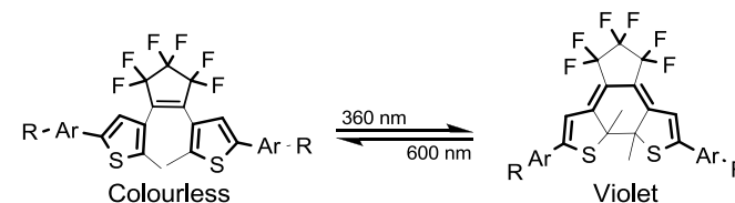
Figure. Photoswitching of a dithienylethene photochromic molecule from an open form to a closed form.
