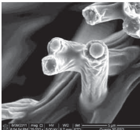
Figure 1. SEM photographs of PGS/PLLA core/shell fiber
