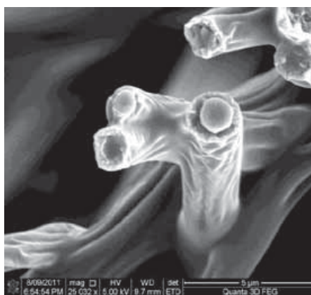
Figure 2. SEM of PGS/PLLA core/shell fiber
