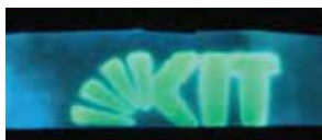
Figure 1. Pattern of PMMA on cellulose obtained by light-induced 1,3-dipolar cycloaddition
